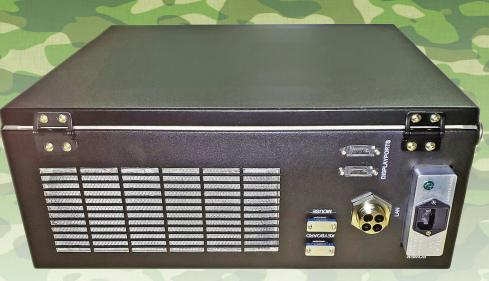
Turnkey systems typically include (but are not limited to) an Intel<sup>®</sup> i7 processor, ATX motherboard to your specifications, 32 GB memory, storage options, latest Windows<sup>®</sup> operating system, USB 3.0 ports, a card reader for extra security, fiber port options, DB9/DB37 connectors, and high-performance power line filter.
