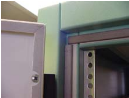
Figure 5 Equipto Electronics FCC cabinet corner showing the metalized door and the gasket configuration.
