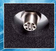
Fiber wave guide as seen from inside the Ka Shield cabinet.
