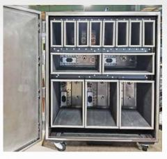
Multiple test compartments with variable shielding effectiveness to simulate interaction between devices in the real world.
