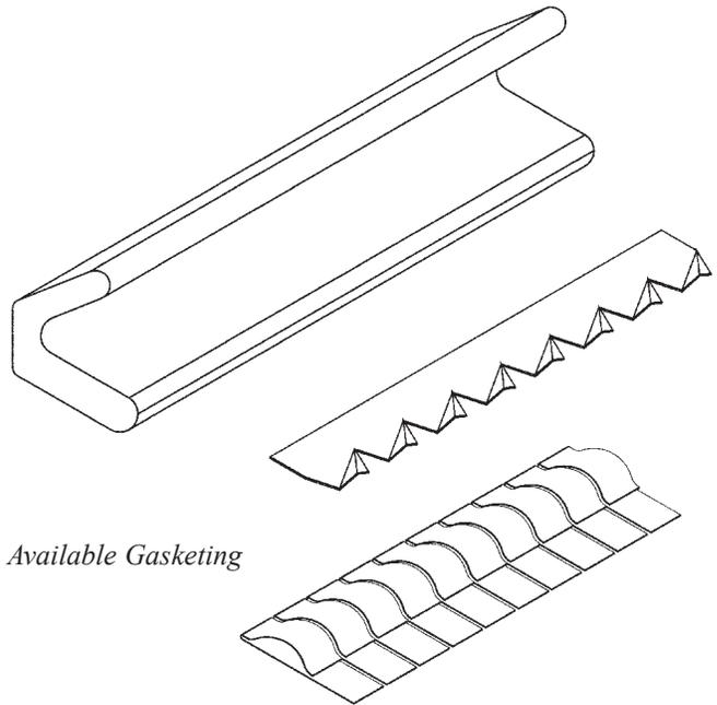
Beryllium copper spring-finger gasketing assures high shielding integrity without requiring adjustment to compensate for a compression set. When double gasketing is required, nickel/copper coated gasketing is added in the compression flange of the frame.
