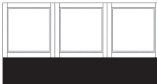
*Triple-width Laminated Plastic Console Shelf attached to three bay cabinet assembly*
