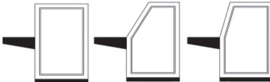
*The three basic cabinet frame types shown above can be joined side-by-side, with Angular Frames to form angular console assemblies*
