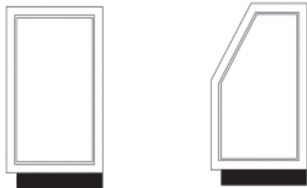
Recessed Pontoon Base has a 4" toe recess in front, flush sides and back
