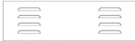
Louvered Flush Filler Panel used to provide for normal venting applications
