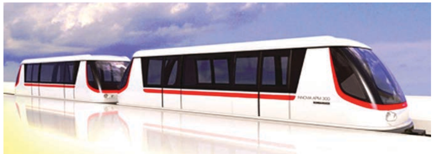
Fig. 1: Bombardier Transportation's INNOVIA APM 300 automated people-mover (APM) system will have cabineted electronics that must operate at 118°F temperatures in Dubai.
